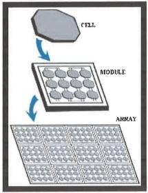
Solar panels are also known as photovoltaic cells. They come in cells, modules, and arrays. Solar panels use light energy from the sun to generate electricity through the photovoltaic effect. The photovoltaic effect is the creation of voltage or electric current in a material upon exposure to light. They are used in some models of airplanes, lasers and vehicles. Scientists also incorporate solar panels into space craft. They use them in space stations and laboratories.
